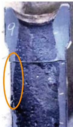
Erosion around the molten steel impact area
